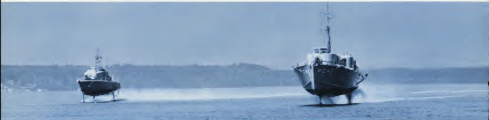
Boeing's high-speed all-weather hydrofoils, TUCUMCARI and HIGHPOINT, are operational with United States Navy.
