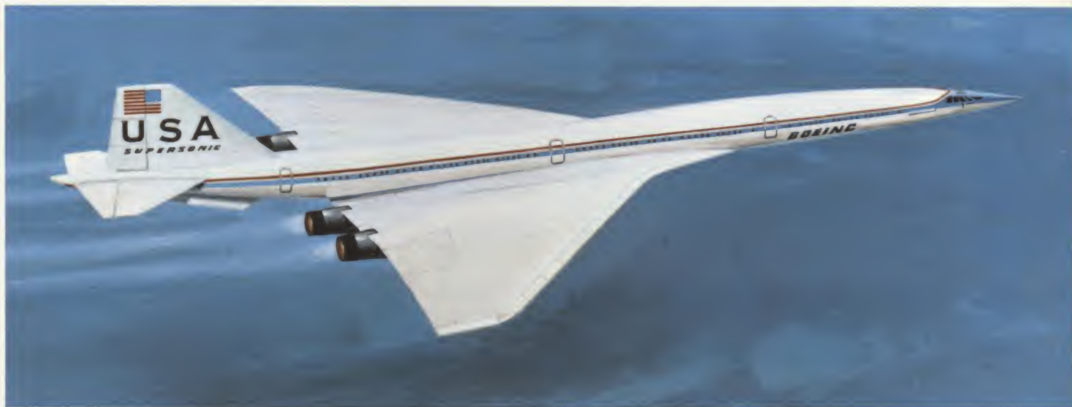
Boeing's proposal for the U.S. Supersonic Transport would carry 300 passengers at 1800 miles per hour.
